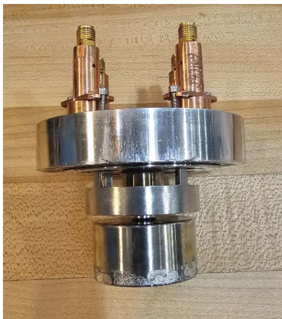
Figure 2-5. The as-built Compact LCM Module, with the four B-dot probes on top.
